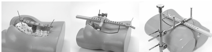
Fig. 14.4 Three platforms allow robotic guidance: a clamp ( left ), the Hover T frame ( center ), and a bed-mount device ( right ). The latter two are for use in minimally invasive spine surgery, while the clamp is used in open procedures
