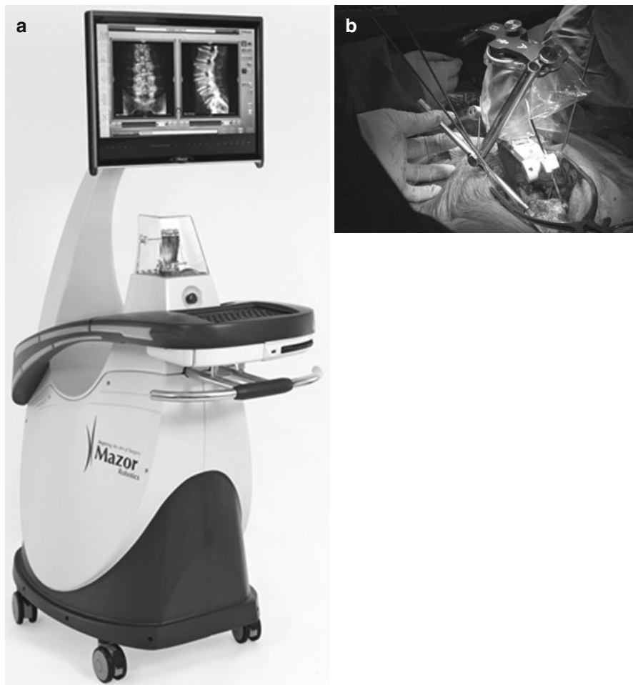
Fig. 14.2 (a) A robotic workstation (Renaissance, Mazor Robotics, Caesarea, Israel). The computer runs software allowing preplanning, image acquisition, registration, and control of robot execution; a touch screen and a 250 g 6 DF miniature robot. (b) The robot is mounted on a clamp, which is connected to a posterior fusion mass in a revision surgery (Photo courtesy Dr. I.H. Lieberman, Texas Back Institute, Plano TX, USA)
