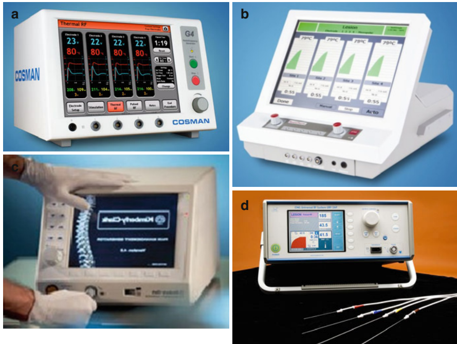
Fig. 3.17 RF Generators (a) The Cosman G4 four-electrode RF generator (b) NeuroTherm NT2000 RF lesion generator (c) Kimberly-Clark Pain Management System (d) Diros OWL URF-3AP Multi-Lesion
