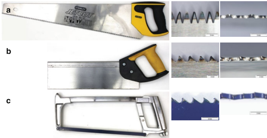
Fig. 4.11 A typical (a) hardpoint, (b) tenon, and (c) hacksaw showing the geometry ( middle column ) and set of the saw teeth ( end column ), respectively. For the hardpoint and tenon saws, the saw teeth are set in a crosscut geometry. The hacksaw has a wavy-set teeth setting
