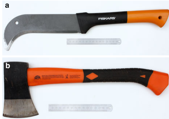
Fig. 4.13 (a) A typical billhook with a fiberglass handle. (b) A typical hand axe with a fiberglass handle
