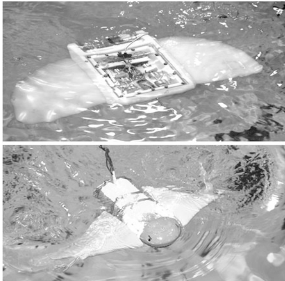
Fig. 12.4 Bioinspired robots (MantaBots) based on the design and swimming kinematics of rays. The mechanical rays were built by Princeton University ( top ) and the University of Virginia ( bottom )
