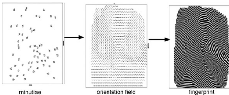
Fig. 8.1 Reconstruction of a fingerprint image from the minutiae template [18]
