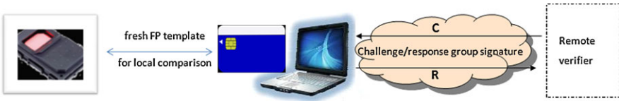
Fig. 11.9 Overview of the authentication phase for the private remote biometric authentication scheme
