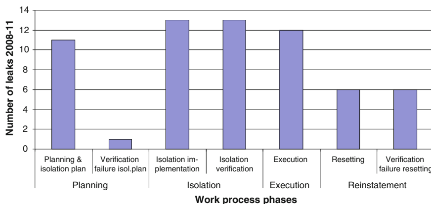
Fig. 6.20 Distribution of errors during leaks due to manual intervention (B and C categories), NCS, 2008–11, for each work process phase separately ( n = 32 ) (Copyright 2012, SPE/APPEA international conference on health, safety, and environment in oil and gas exploration and production drilling conference and exhibition copyright. Reproduced with permission of SPE. Further reproduction prohibited without permission)
