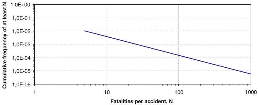
Fig. 2.2 Risk tolerance limit in f-N diagram
