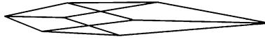
Fig. 2.3 An image of a 3D projective transformation of a cube (from Pizlo [16])
