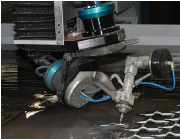
Fig. 6.11 Typical cutting head of Flow MACH 4 4020b AWJ machine [73]
