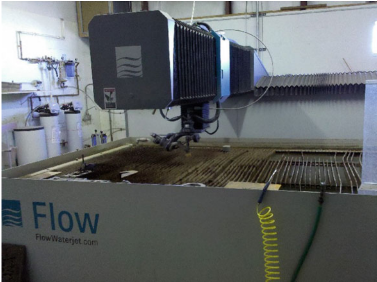
Fig. 6.10 A typical Flow MACH 4 4020b AWJ machine [72]
