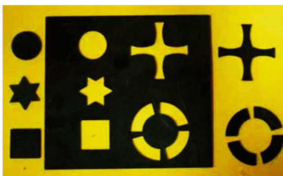
Fig. 1.7 Profile laser cutting carried out at RRCAT
