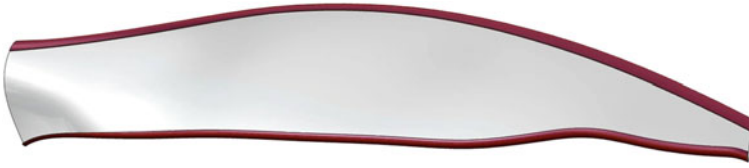
Fig. 7.15 Leading and output edges of the propeller blade
