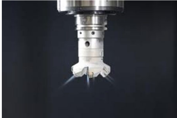
Fig. 7.16 Cryogenic system by Global Retool Group ®
