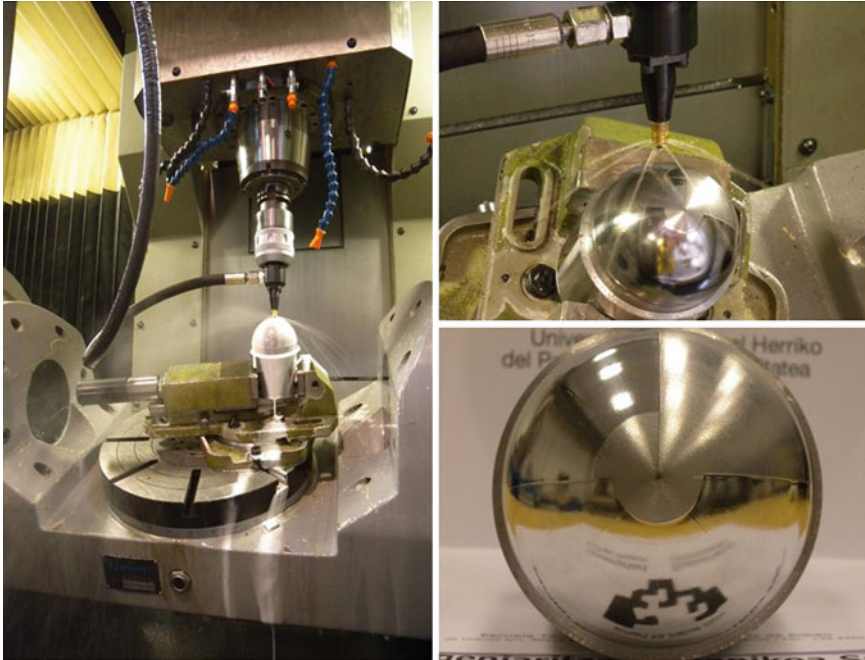
Fig. 7.14 Test piece. ( Left ) Burnishing system in 5-axis machine. ( Up ) Detail of the burnishing tool. ( Down ) Detail of the hemisphere burnished with different strategies (López de Lacalle et al. [21])
