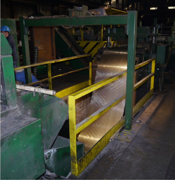
Fig. 7.5 Mechanical setup of the exit loop between the slitter and the recoiler
