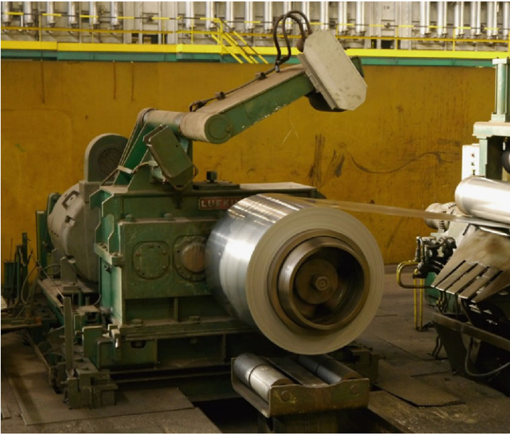
Fig. 7.3 Mechanical setup of the uncoiler (150 kW DC drive)
