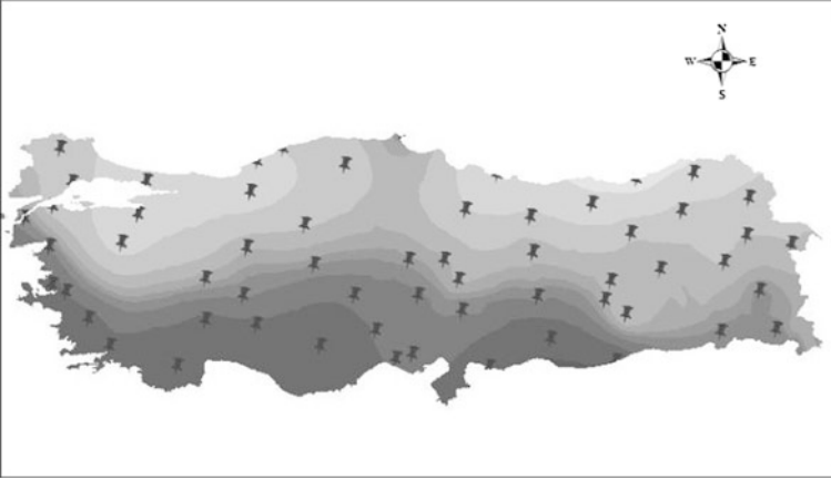
Fig. 6.3 Meteorological measurement stations and kriging prediction surface for solar radiation: the case of Turkey
