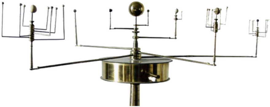
Fig. 10.11 In this mechanical orrery by Gilkerson, housed in the Armagh Observatory the movement of the planets and their moons are mechanically simulated. It is not possible to access an arbitrary position of the system without moving through intermediate states. This is a feature of simulation systems: they do not have a closed form or analytic solution. To compute the state of the system at t_{12} one must determine the state at t_{11} and move from there
