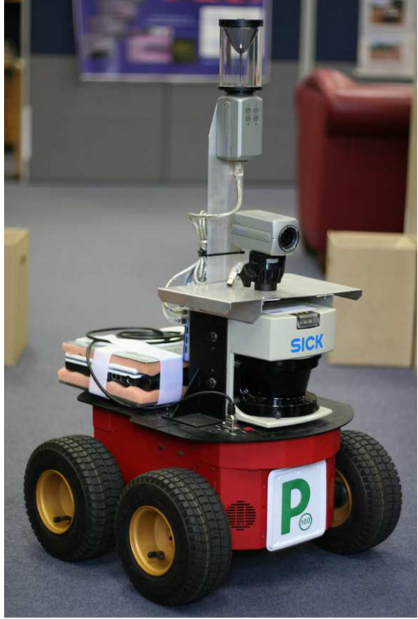
Fig. 5.4 Typical mobile robot equipped with a bearing only sensor (vertically mounted panoramic camera)
