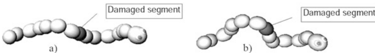
Fig. 6.16 The frontal view of the Snakebot before (a) and after the adaptation (b) to the damage of single segment. The corresponding views from above of the sidewinding Snakebot are shown in Fig. 6.15a and 6.15b respectively
