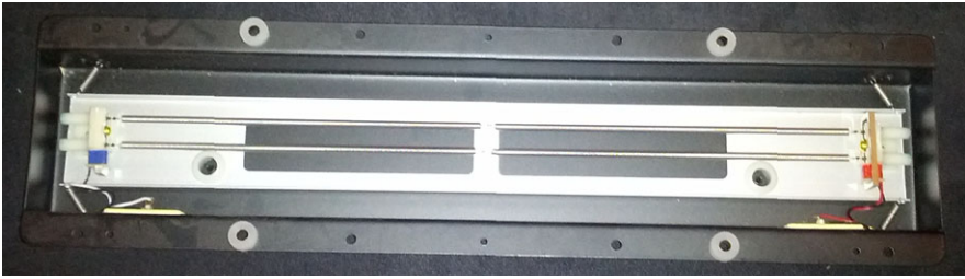
Fig. 9.24 Mechanical spring-based delay unit. An analog signal can be sent into one end of this unit, where it is transformed into mechanical motion that causes the springs to oscillate. The signal travels through the spring to the other end, where a transducer converts the mechanical motion back into an electrical signal, which can be amplified and re-sent to the starting point. This is one way to store an analog signal
