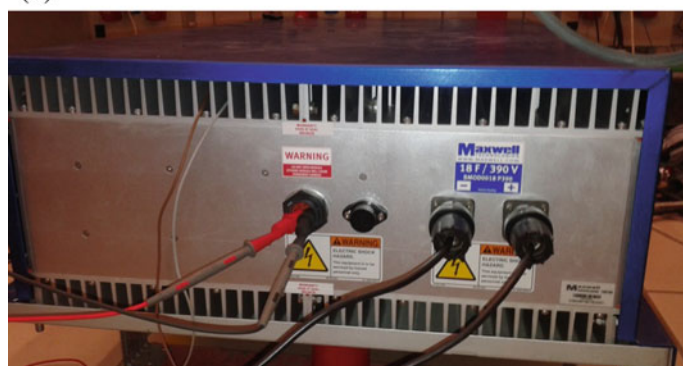
Fig. 10.2 EDLC technology. a Basic cells structure. b 18F/380 V EDLC stack under test at the ESD-Lab sited in the Engineering School of Seville's University
