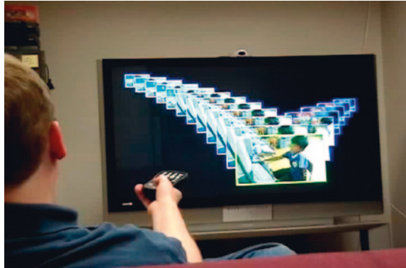
Fig. 1.16 An interface designed to facilitate fast-forwarding and rewinding by providing context. The speed of movement can be controlled manually (courtesy of Kent Wittenburg)
