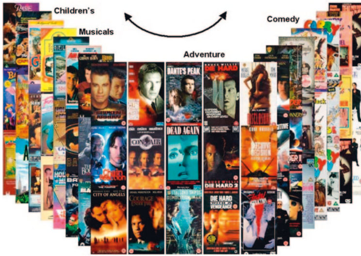
Fig. 1.15 A video store: movement of a cursor along the ‘walls’ causes posters to pop out. The bifocal arrangement of the wall is such that a click on a full view causes a short movie illustrating the video to be shown (reprinted from Spence 2007)
