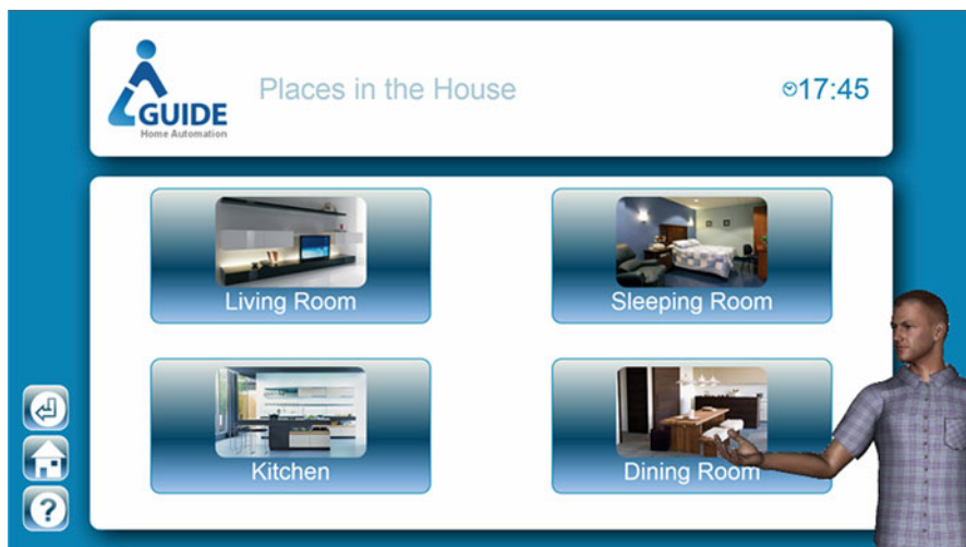
Fig. 7.1 An EVA being developed in the GUIDE project [55] that uses gestures to accompany short verbal presentations
