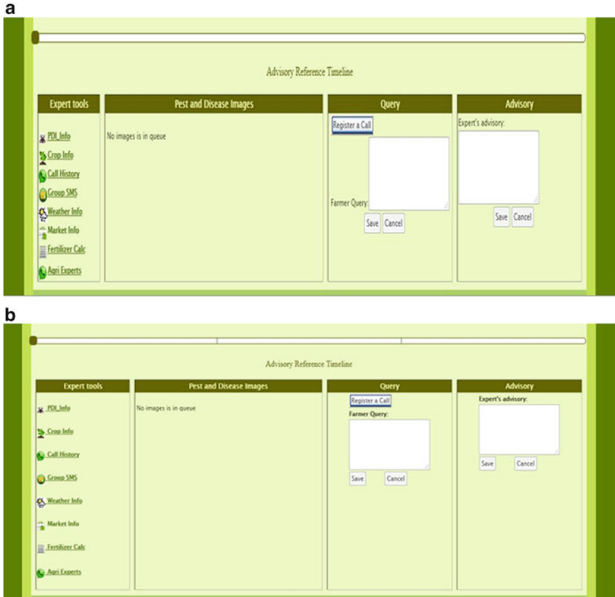
Fig. 4.12 Application of the user model. (a) Previous inter-button spacing and hyperlink spacing. (b) Modified inter-button spacing and hyperlink spacing
