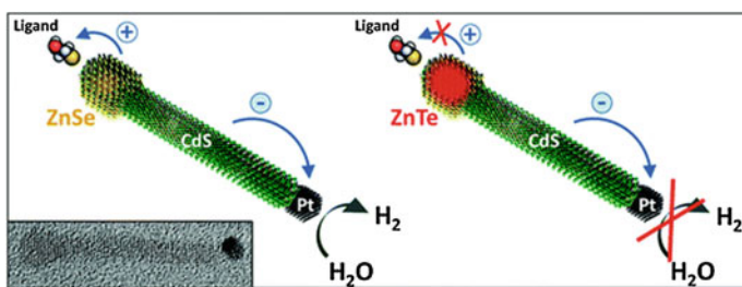
Fig. 17.1 Scheme showing the different behaviour for water splitting of ZnSe/CdS/Pt heteronanostructures when the surface is unmodified ( right side ) or stabilized with electron donor molecules ( left ). The inset at the bottom shows the high-resolution image of one of these nanostructures. Reproduced with permission from Acharya et al. 2011. Copyright American Chemical Society
