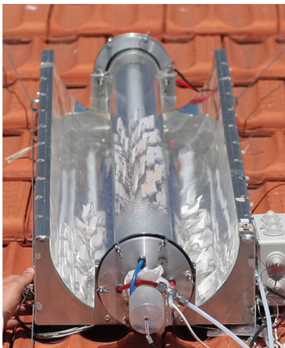
Fig. 3.5 Solar/lamp photocatalytic reactor for gaseous H 2 S elimination field test at a wastewater treatment plant in Madrid (Spain). Design and photography by Benigno Sánchez (Ciemat). Reproduced with permission
