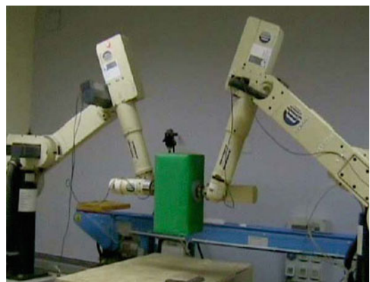
Cooperative Manipulators, Fig. 1 An example of a cooperative robotic work cell composed by two industrial robot arms
