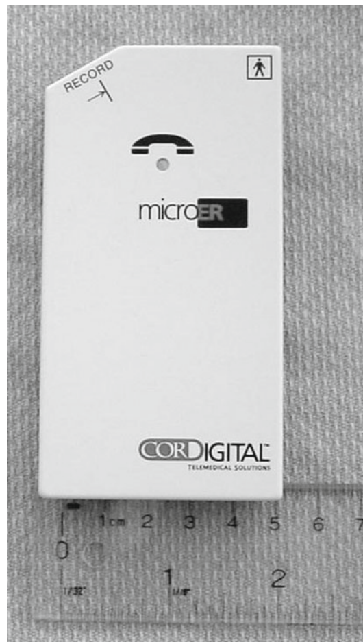
FIGURE 15–2. Transtelephonic Monitors. The device is lightweight and portable, easily placed in a handbag or pocket. Four recording electrodes are present on the back of the device to permit single lead rhythm strip capture. A record button ( top left ) is pressed in the event of symptoms, and the recorded event is transmitted to a base station over an analog phone line
