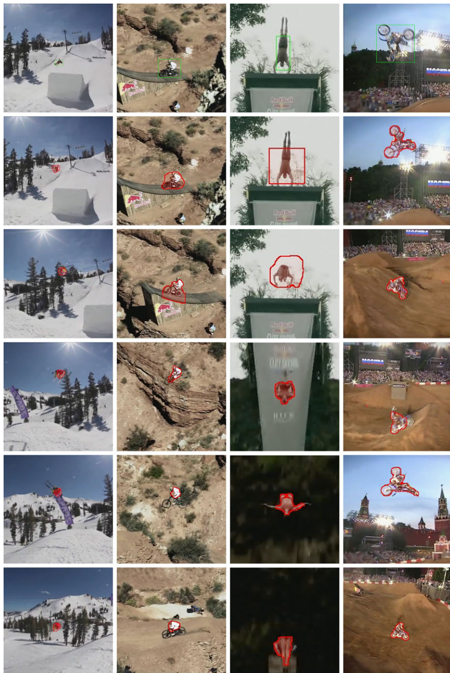
Fig. 12.5 Illustrative tracking results. Manual initialization ( first row ) and selected frames ( row 2 to 6 ) from several sequences. ( Green : initialization rectangle; red : tracking result)
