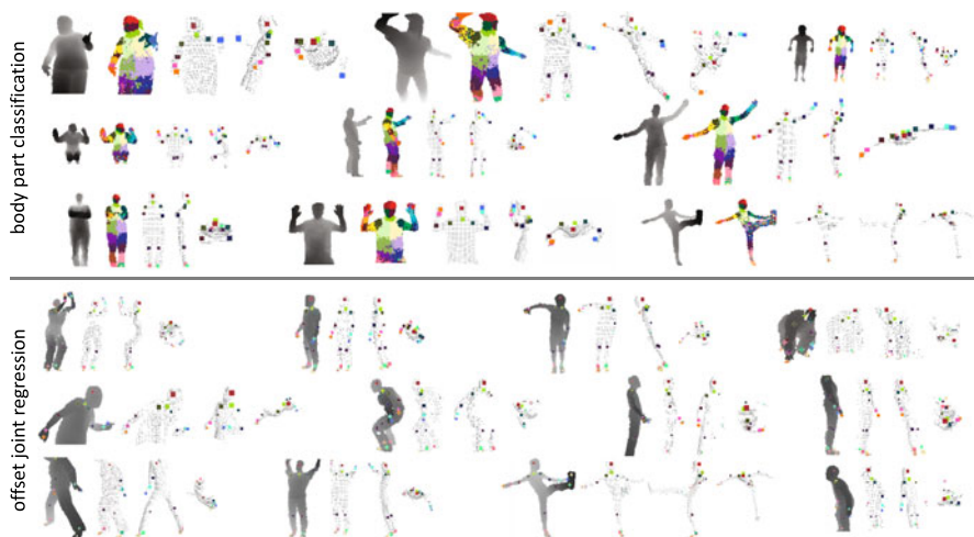
Fig. 13.6 Example inferences on both synthetic and real test images. In each example we see the input depth image, the inferred most likely body part labels (for BPC only), and the inferred body joint proposals shown as front, right, and top views overlaid on a depth point cloud. Only the most confident proposal for each joint above a fixed, shared threshold is shown, though the algorithms predict multiple proposals per joint. Both algorithms achieve accurate prediction of body joints for varied body sizes, poses, and clothing. We show failure modes in the bottom rows of the two panels. There is little qualitatively to tell between the two algorithms, though the middle row of the OJR results shows accurate prediction of even occluded joints (not possible with BPC), and further results in Sect. 13.4.3 compare quantitatively
