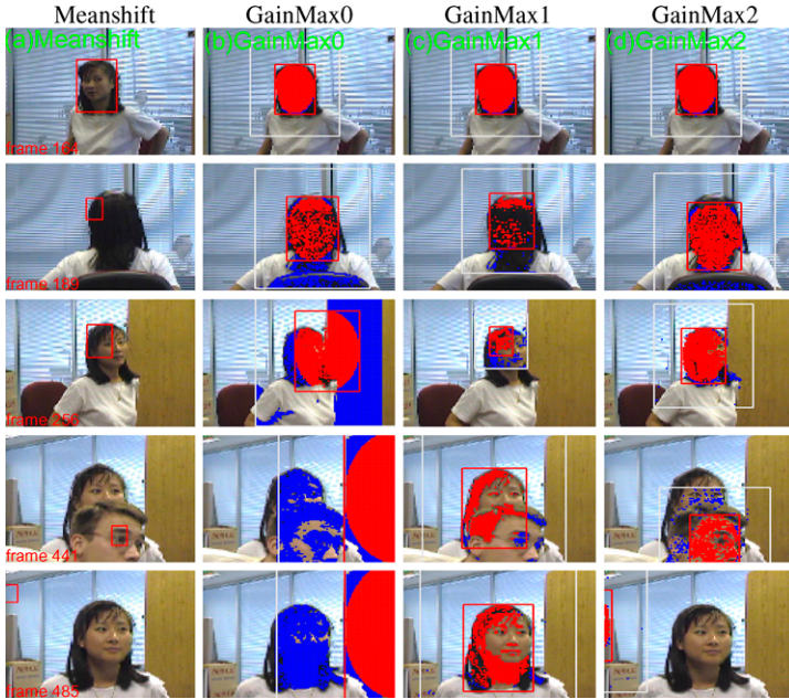
Fig. 19.8 GainMax trackers using gradient ascent information gain maximization can handle distraction and occlusions well. For the mean-shift tracker (column 1), the red box is the tracking result; for GainMax trackers 0–2 (columns 2–4), red indicates pixels correctly labeled in the ellipsoid as target (true positive), blue indicate false positive pixels outside of the target ellipsoid
