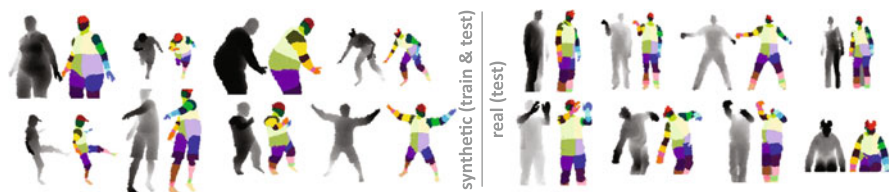
Fig. 13.2 Synthetic vs. real data. Pairs of depth images and corresponding color-coded ground truth body part label images. The 3D body joint positions are also known (but not shown). Note the wide variety in pose, shape, clothing, and crop. The synthetic images look remarkably similar to the real images, lacking primarily just the high-frequency texture
