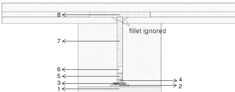
Fig. 11.3 Cross-section split into elements for moment resistance calculation. From Sha (2001b)
