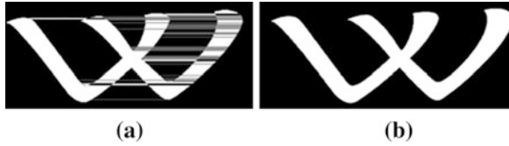
Fig. 16.4 Filling the area for high-accuracy a the point spacing of the Gerber files record is less than the threshold b achieve the purpose of rasterization
