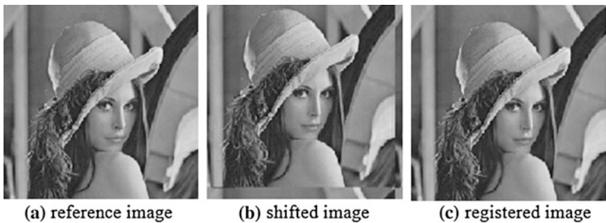
Fig. 64.2 Reference images (a), the object image (b), and after shifted (15.658, 10.345) and the registered image (c) with \lambda = 100
