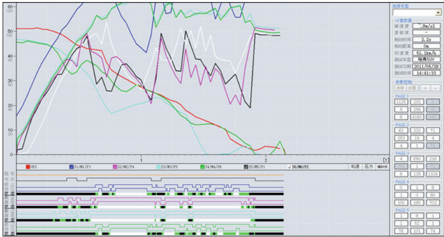
Fig. 73.3 Emergency straight braking performance of HaFo-H3 ABS (on dry concrete road, initial speed = 50 km/h)
