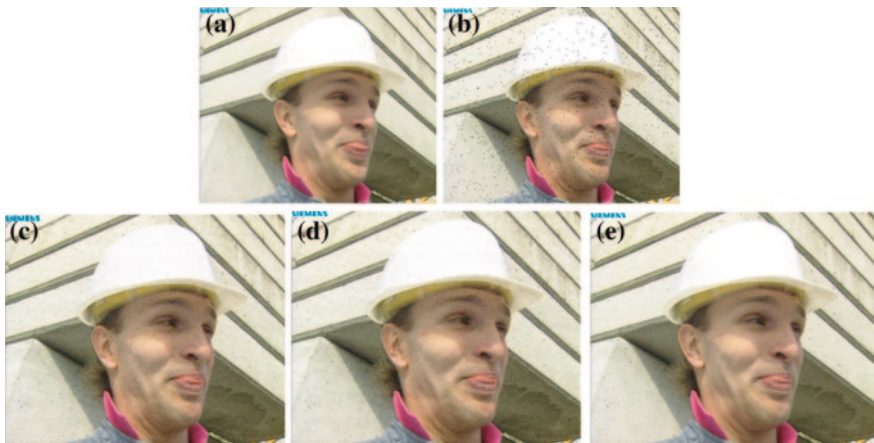
Fig. 69.1 The seventh frame image of forman: a image after salt and pepper noise experienced pre-filtering; b image with 24 dB salt and pepper noise; c image after Gaussian noise experienced pre-filtering; d image with 32 dB Gaussian noise; e original image
