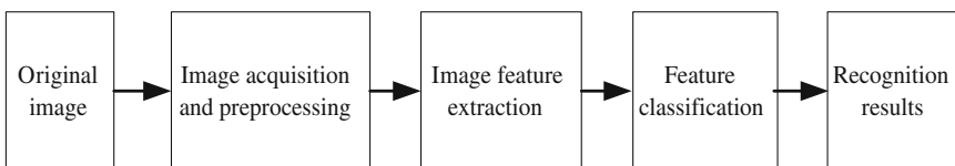
Fig. 96.1 The structure of the image recognition system
