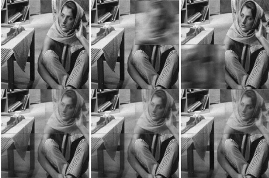
Fig. 101.3 Image Fusion comparisons for Barbara image. a Clean image, b upper right blurred, c lower left blurred, d average fusion, e wavelet fusion, f QSVD fusions
