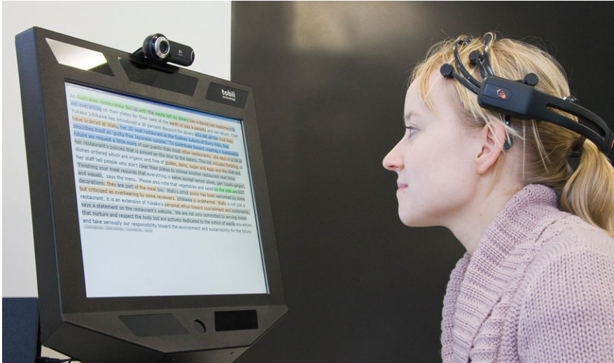
Fig. 8.8 For the emotion measurement we make use of a low cost EEG device. While the user works on the eye tracker muscular activity and brain waves are also recorded and stored with the gaze data for real-time reaction and later analysis
