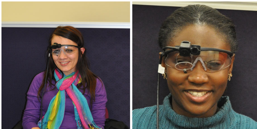
Fig. 4.1 ASL MobileEye gaze tracking systems were worn by both conversation partners during the experiment
