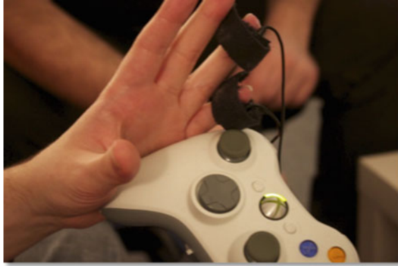
Fig. 27.2 GSR sensors fitted to the player's hand to capture arousal during gameplay
