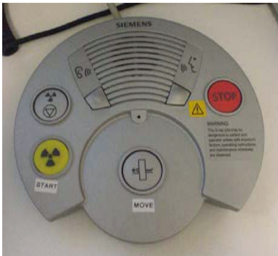
Fig. 13.5 Additional operating and voice intercom system utilized for the CT aspect of a SPECT/CT study
