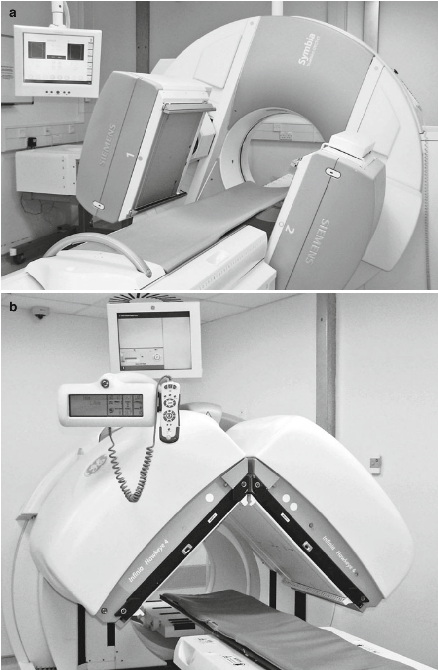
Fig. 4.5 Typical SPECT-capable gamma cameras. (a) Siemens Symbia, shown with the two detectors in H-mode. (b) GE Infinia, shown with the two detectors in L-mode
