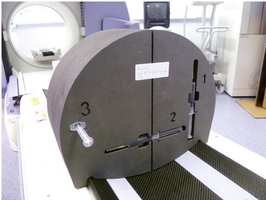
Fig. 6.17 SPECT-CT alignment check setup for GE Hawkeye
