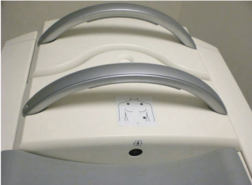
Fig. 6.13 Integrated ECG port on the patient imaging pallet allows seamless acquisition of cardiac gating data during myocardial perfusion examinations
