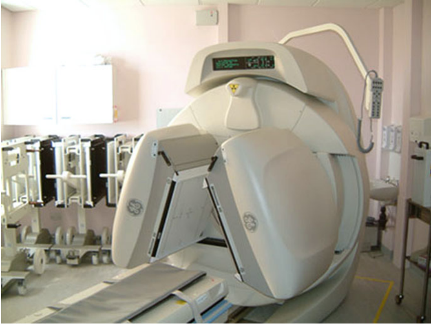
Fig. 6.6 GE Hawkeye SPECT/CT system, with integrated X-ray unit, consisting of a low-output X-ray tube and cadmium tungstate detectors
