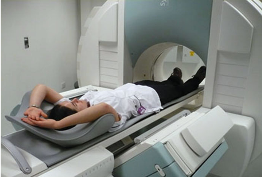
Fig. 6.12 Variable geometry of gamma camera heads on a modern SPECT/CT system, reducing the “closed” space during the CT procedure
