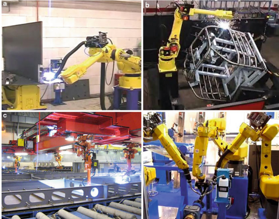
Fig. 1 Examples of robotic welding: (a) welding a workpiece on a turntable ( www.forster-welding-systems.com ), (b) welding a car frame ( www.lincolnelectric.com ), (c) robot panel welding for shipyard automation ( www.kranendonk.com ), (d) arc welding station with two welding robots and one workpiece handling robot ( www.forster-welding-systems.com )
