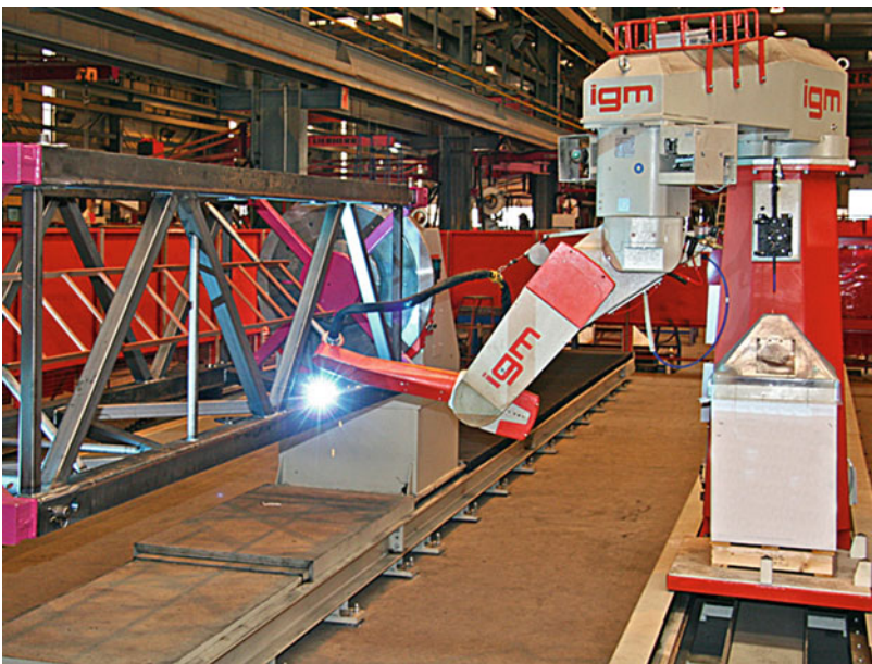
Fig. 15 Column-mounted welding robot ( www.igm-group.com )
