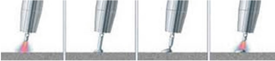
Fig. 7 Illustration of the hot and cold periods during CMT
