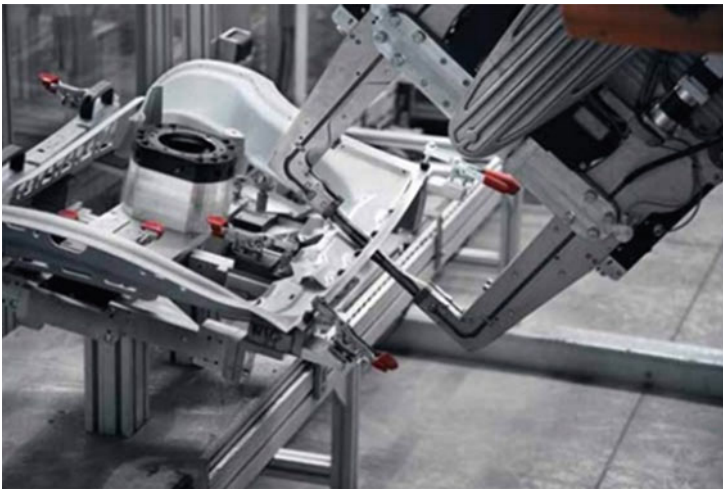
Fig. 4 DeltaSpot for joining a 1.5 mm thick stiffening plate onto a 2 mm thick die-cast aluminum door frame
