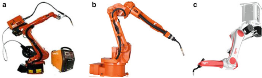
Fig. 21 Welding robot arms, (a) robot with a welding power source, (b) arm with hollow wrist for cables, (c) ceiling mounted robot
