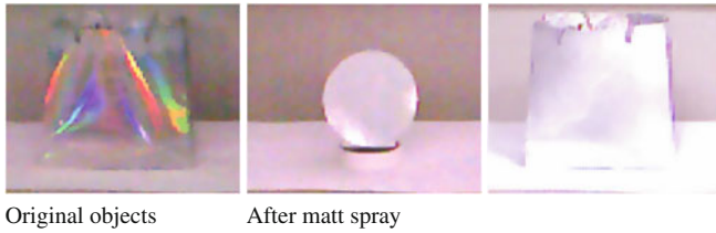
Fig. 1.14 We apply white matt spray on top of non-Lambertian objects for ground truth depth acquisition. Original objects after matt spray
