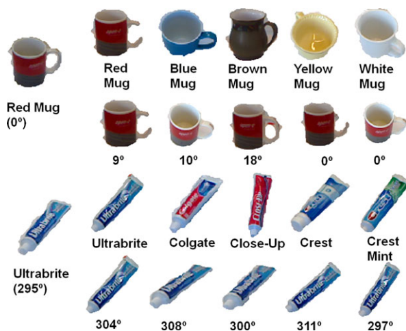
Fig. 9.7 Recognition results from the Object-Pose Tree for two objects: Red Mug (top left), and Ultrabrite Toothpaste (top right). (Bottom) From left to right, the top five objects with the highest classifier response at the instance level and at the pose level for Red Mug and Ultrabrite toothpaste
