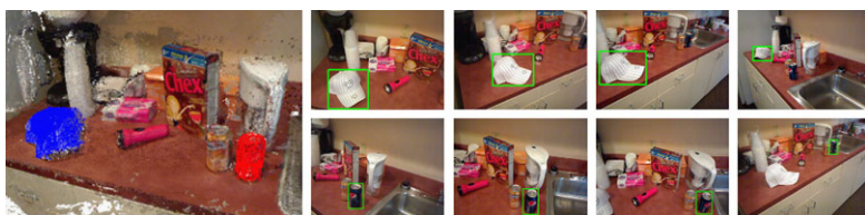
Fig. 9.5 (Left) 3D scene reconstruction of a kitchen scene with a cap highlighted in blue and a soda can in red using the labeling tool. (Right) Ground truth bounding boxes of the cap (top) and soda can (bottom) obtained by labeling the reconstruction
