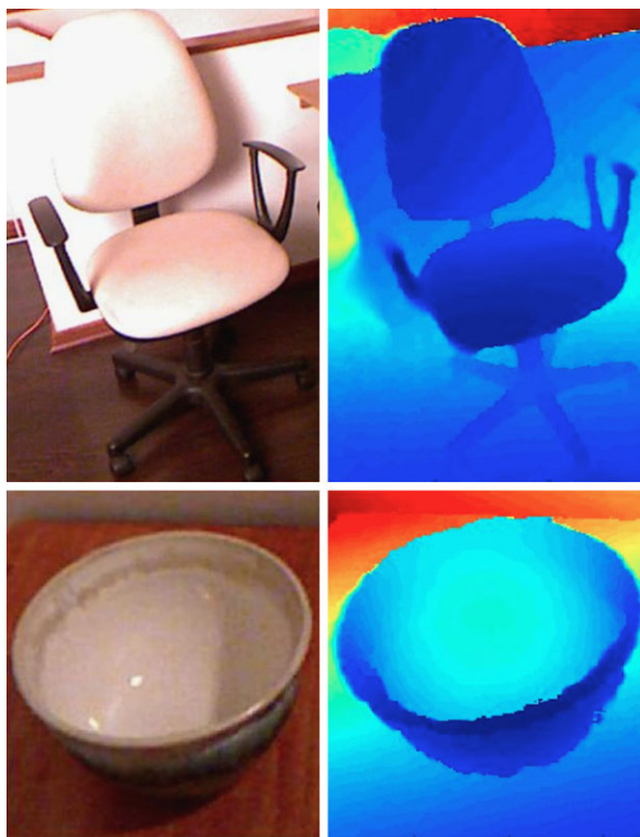
Fig. 8.2 The office chair on top illustrates an example where the depth discontinuities identified by HOG on a depth image would offer additional information not as easily identified from the intensity image. The bowl on the bottom shows an example where gradients on the depth image would not be expected to yield much that could not be understood from the intensity image
