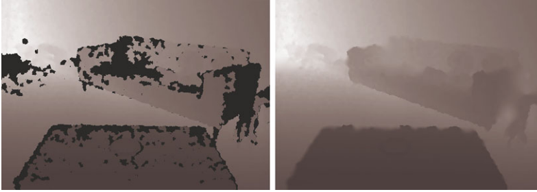
Fig. 8.4 Illustration of our depth smoothing method. The original depth image is shown on the left where black pixels demonstrate missing depth data. The smoothed image is shown on the right
