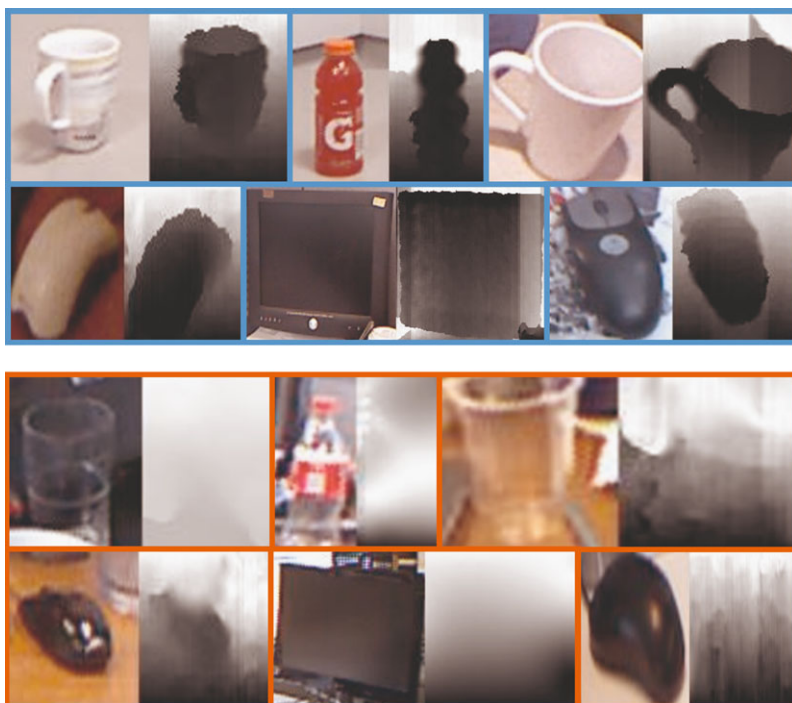
Fig. 8.8 The top two rows of images show examples of good depth data for various objects. The bottom two rows show examples of missing depth data for objects of the same classes as shown in the top two rows . All examples illustrate depth after smoothing as described in Sect. 8.3.3
