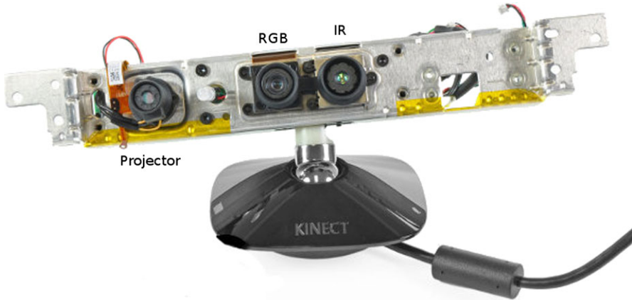
Fig. 1.1 Kinect consists of infrared (IR) projector, IR camera and RGB camera (illustration from [11])
