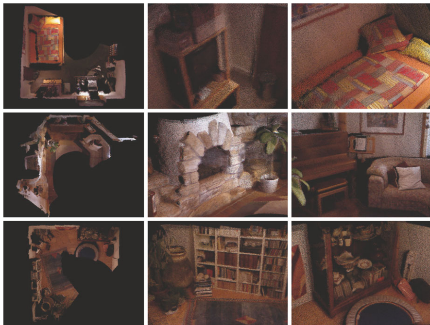
Fig. 2.6 On-the-fly 3-D scene reconstruction for different types of room. First row : bedroom (295 frames). Second row : lounge (526 frames). Third row : family room (380 frames). For each sequence, the left column depicts a bird-eye view of the respective room layout. The remaining columns provide a zoom-in for selected regions. All reconstructions were performed using our default parameter settings as stated in Sect. 2.5.1. Note that for visualization of the reconstructed scenes, we rendered a subset of the global model point cloud
