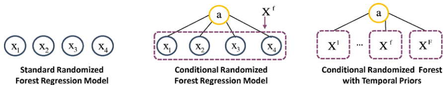
Fig. 4.3 The figure shows the relationships encoded by different regression forest models. The basic model ( left ) makes predictions for each body joint independently. The conditional model ( center ) encodes dependency relationships between the body joint positions and a global variable. The temporal conditional regression forest model ( right ) incorporates the prior that the value of the global variables associated with multiple image frames should be consistent. For instance, the height of a human subject remains constant through the video sequence
