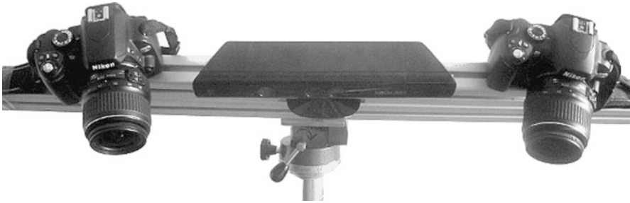
Fig. 1.2 A rig with a Kinect and two Nikon D60 SLR cameras
