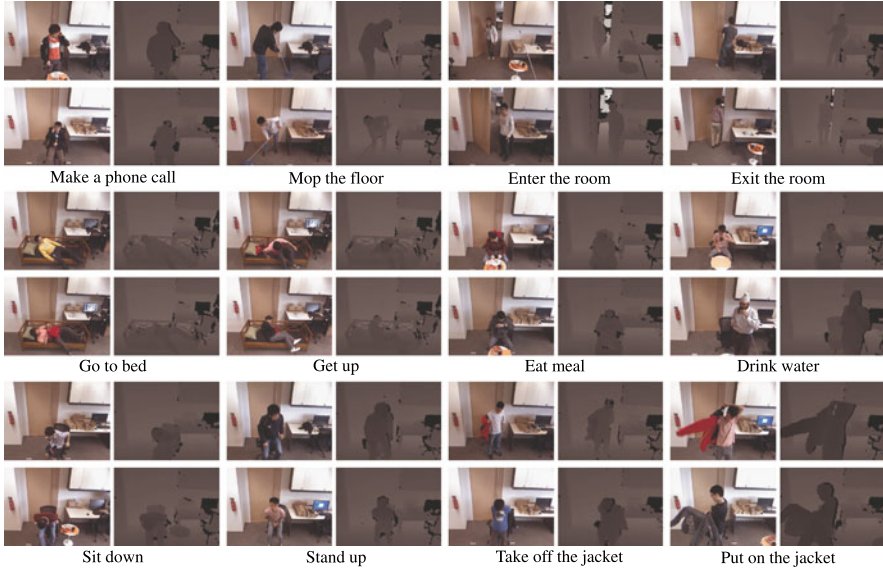
Fig. 10.2 Example color and depth frames from each activity category. Note for the depth map, brighter pixels mean larger depth values. Some black regions correspond to depth measurement errors due to surface reflections, i.e., the PC screen
