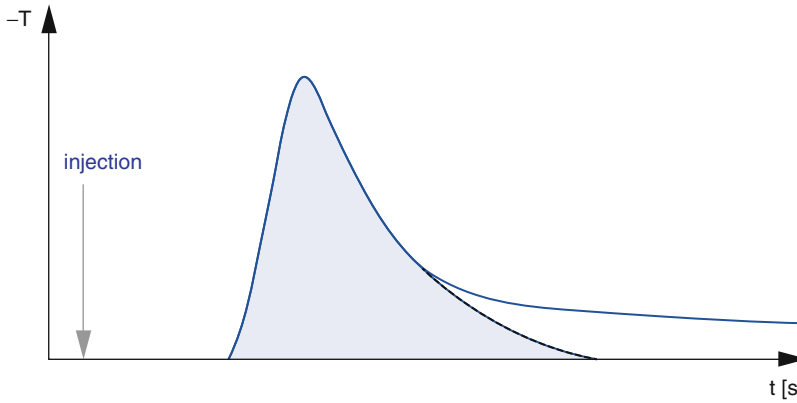
Fig. 50.1 A thermodilution curve from a transpulmonary cardiac output monitoring device: the period from indicator injection to measurement of curve represents the transit time. The dilution curve indicates the measured change in temperature over time (an equivalent curve would be
