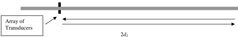
Fig. 15.4 Second part of the pulse-echo movement and d_2
