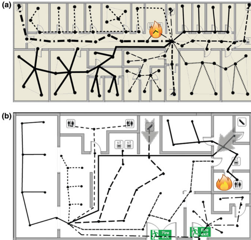
Fig. 1 Two floor plans of the three-storey building simulated. The graphics show the sensor nodes ( black dots ) and the network layout (each zone marked with a different line style), and the fire outbreak locations in each scenario ( flame icon ). a Floor 2; b floor 1
