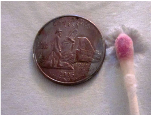
FIGURE 2.10 Positive nickel confirmatory test using 1 % dimethylglyoxime-ammonia (DMG-A), which turns pink upon contact with nickel items
