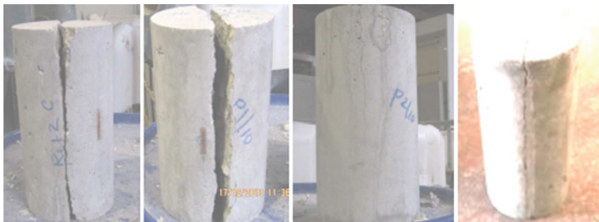
Fig. 4.35 Concrete specimens after the determination of tensile splitting strength, from left to right: concrete with natural, pellet-shaped PET, fine and coarse PET flakes aggregates (Saikia and de Brito 2010)
