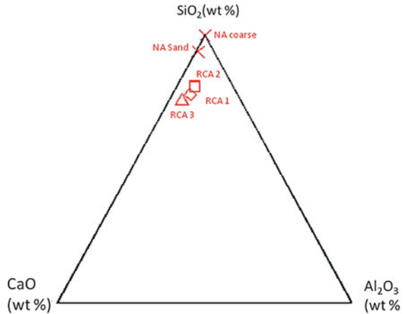
Fig. 3.17 Position of natural aggregate (NA) and CDW aggregates (RCA) in CaO-SiO 2 -Al 2 O 3 ternary diagram (Limbachiya et al. 2007)
