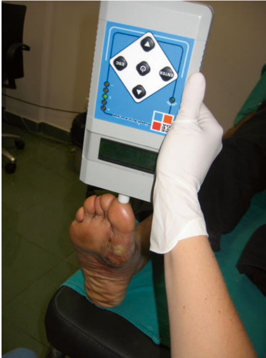
FIGURE 5.2 The measurement of vibration perception threshold on the toe of a diabetic patient
