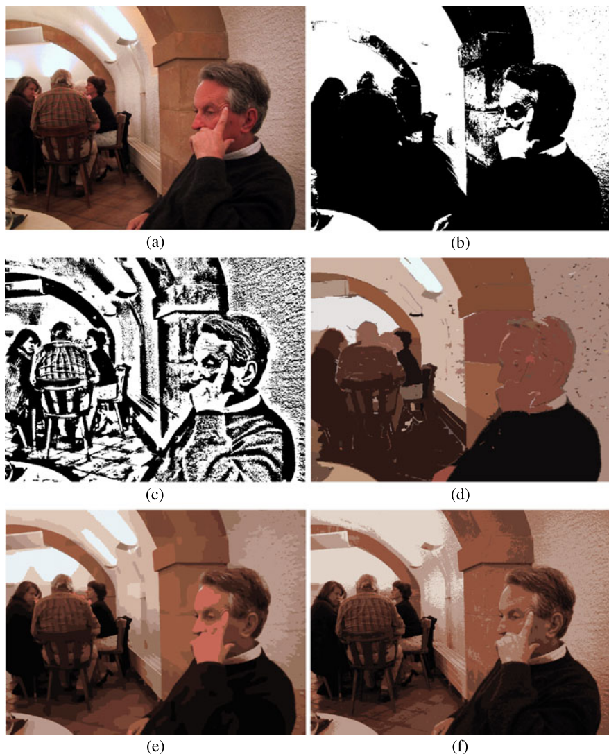
Fig. 11.2 Unsuccessful attempts to render images using computer vision algorithms. (a) Source colour image (courtesy of Anthony Santella), (b) image with global thresholding, (c) image with local thresholding, (d) segmented image with regions rendered with the mean colour from the corresponding source colour image pixels, (e) alternative segmentation, (f) image with colour quantisation using median cut (10 colours)
