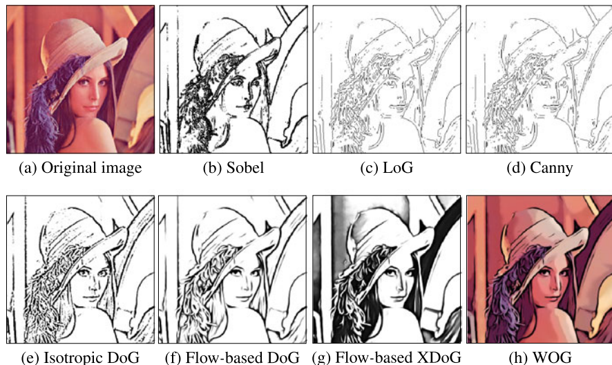
Fig. 5.5 Example showing the output of different edge detection and stylization methods. (a) The original image (USC-SIPI image database). (b) The globally thresholded gradient magnitude of the Sobel filter. (c) Zero-crossing of the Laplacian of Gaussian [40]. (d) The output of the Canny edge detector [11]. (e) The thresholded DoG as proposed in Winnemöller et al. [60]. (f) The thresholded output of the separable implementation of the flow-based DoG [26, 31]. (g) The flow-based DoG with XDoG thresholding. The image is pre-processed with a bilateral filter to suppress noise. (h) Cartoon-style abstraction generated with bilateral and flow-based DoG filters using the WOG-pipeline
