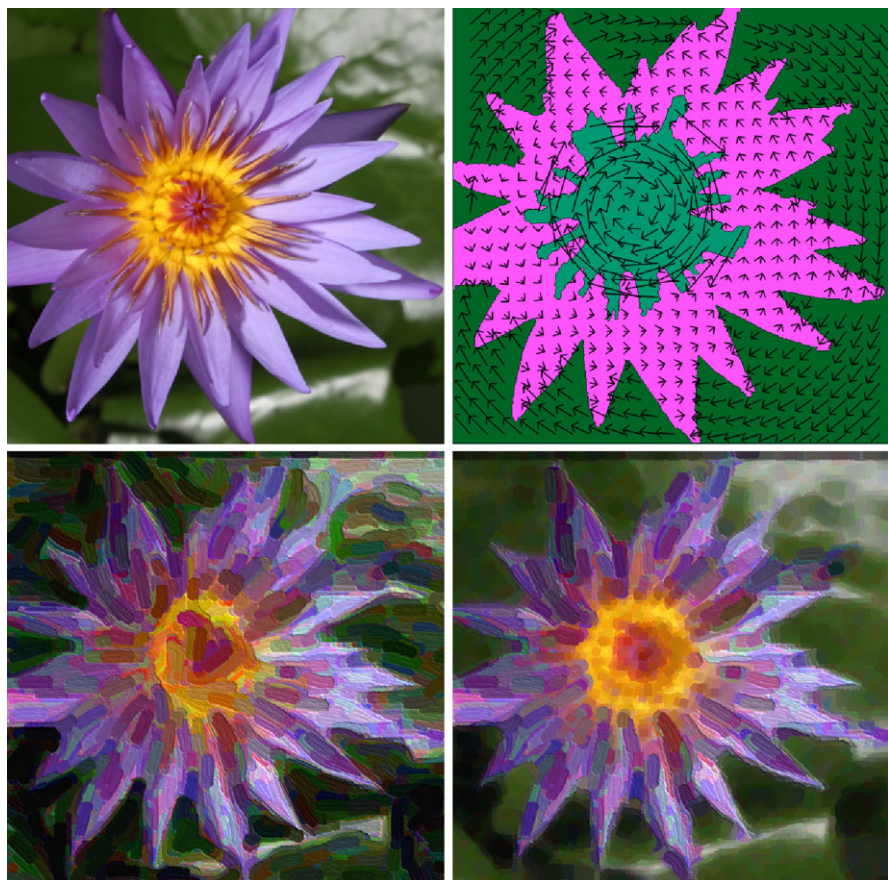
Fig. 6.7 A comparison between single style ( lower-left ) and multi-style ( lower-right ) rendering for input image of a flower ( upper-left ). Notice that in the multi-style rendering, the stamens are given fine details, the leaves are deemphasized, and the contrast between three regions are made more pronounced
