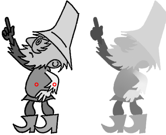
Fig. 14.10 Enforcing smooth depth transitions—the initial depth map ( left ) produced by Lazy-Brush (Sect. 14.2) and the topological sorting algorithm (Sect. 14.3.1) contains artificial depth discontinuities at pixels where the body and arm connects. This artifact can be removed ( right ) by calculating a smooth transition between the endpoints ( red dots ) of the original depth inequality which was used to specify depth ordering of these two regions (depicted in Fig. 14.8). Reproduced with kind permission from Blackwell Publishing Ltd. © UPP & DMP + © EG & Blackwell. Used with permission
