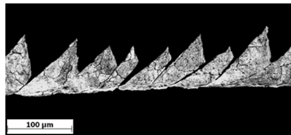
Fig. 6. Microstructure of Ti-676-0.9 alloy chips, v_c = 40 m/min, a_p = 0.5 mm, f = 0.1 mm/rev. The material separations in the primary shear zones are clearly visible.
