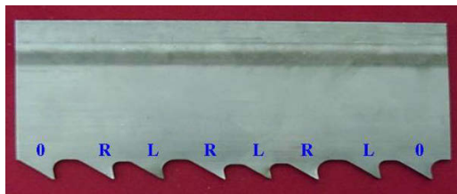
Fig. 1. Bandsaw (1.4/2 TPI) teeth used in this investigation
