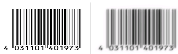
Fig. 1. left: image definition without safety glasses; right: image definition with safety glasses conform to DIN EN 166 (simulation)
