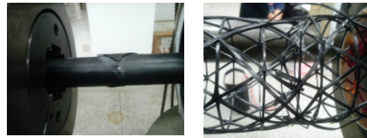
Fig. 5. Torsion specimen damage
