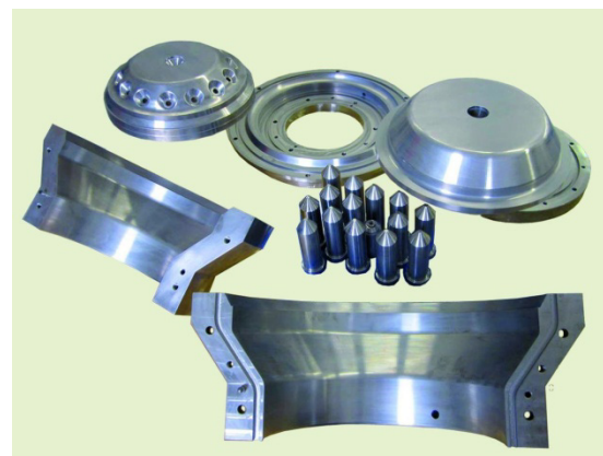
Fig 4. Elements of the casting mold for the first rotor prototypes.
