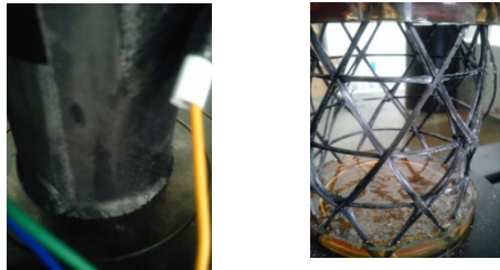
Fig. 3. Compression specimen damage
