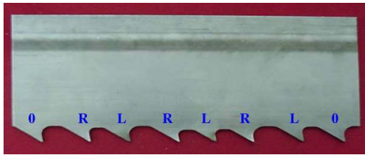
Fig. 1. Bandsaw (1.4/2 TPI) teeth used in this investigation
