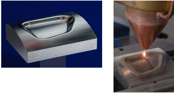
Fig. 5. Part, welding area und process photo.
