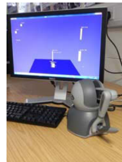
Fig. 2. Virtual Environment including Haptic Device
