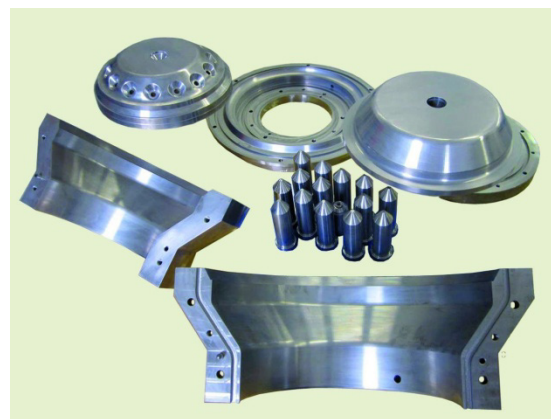
Fig 4. Elements of the casting mold for the first rotor prototypes.
