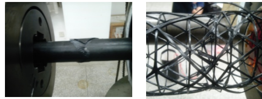
Fig. 5. Torsion specimen damage
