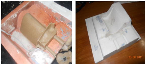
Fig 5. Wax pattern through Plaster Mold
