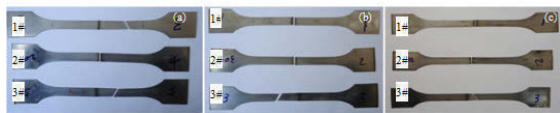
Fig. 3. Images of stretched samples at (a) 200 °C, (b) 300 °C and (c) 400 °C
