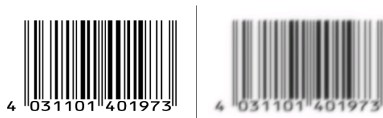
Fig. 1. left: image definition without safety glasses; right: image definition with safety glasses conform to DIN EN 166 (simulation)
