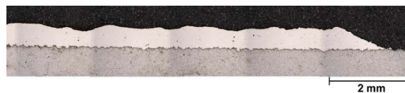
Fig. 9. micrograph showing Stellite 6 coating
