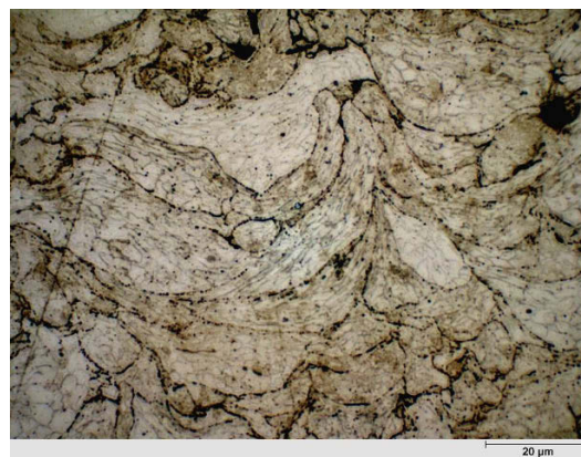
Fig. 8 316L coating etched with marbles reagent
