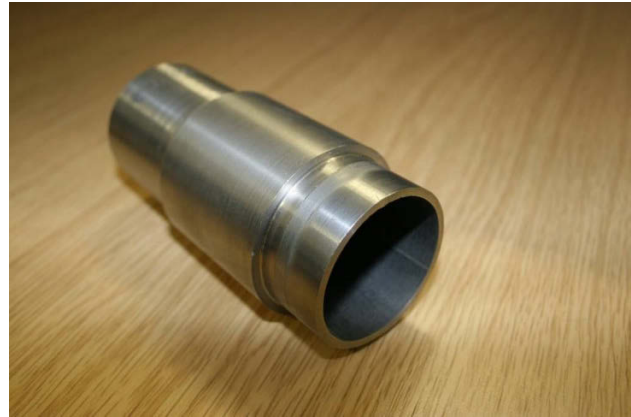
Fig. 5 Thick titanium coating on 51 mm diameter mild steel tube. Shown after post deposition machining.
