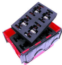
Fig. 1. Soft material packaging example for mass produced parts
