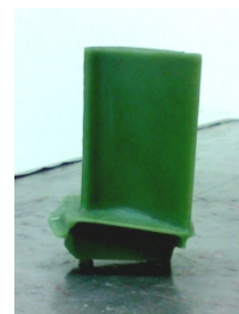
Fig 3. Wax pattern of turbine blade through RTV silicon Mold
