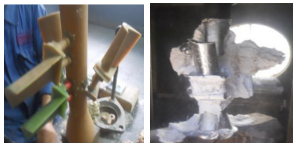
Fig 6. Investment casting of parts
