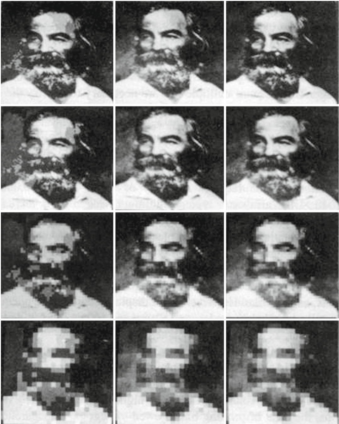
Fig. 5.3 Demonstration of how varying the number of pixels and the number of bits per pixel affects the spatial and contrast resolution of a digital image. The image in the upper right corner was displayed using a 256 x 256 array of pixels, 8 bits per pixel; the subject (Walt
