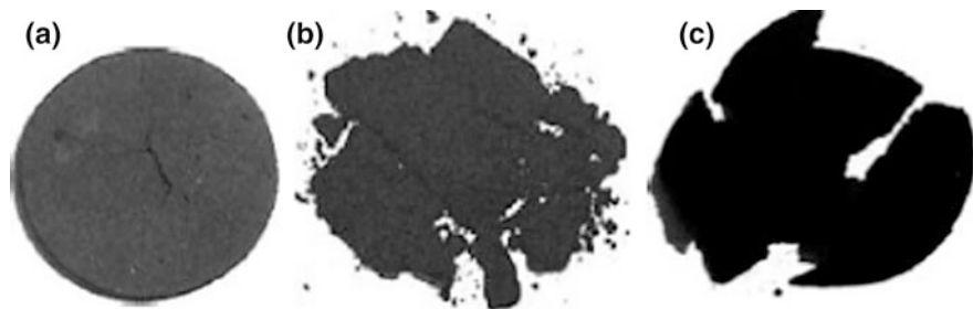
Fig. 6 Photographs of an Ni–YSZ cermet a after heating in H_2 at 800\text{ }^\circ\text{C} , b after heating in 100\% CH_4 at 800\text{ }^\circ\text{C} for 1.5\text{ h} , and c after heating in 40\% toluene at 700\text{ }^\circ\text{C} for 1.5\text{ h} . From Gorte and Vohs [45]. Reproduced here with kind permission from © Academic Press 2003
