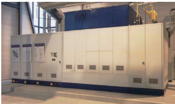
Fig. 9 Siemens Westinghouse's 100 kW SOFC cogeneration system
