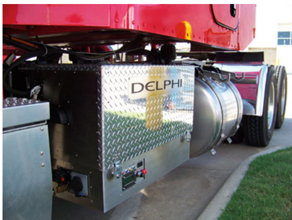
Fig. 13 Delphi's SOFC APU mounted underneath a Peterbilt's truck cabin
