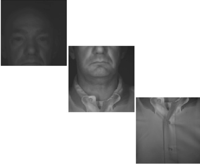
Fig. 12.2 Example of corresponding frames from the IOM as the subject passes through the in-focus region of the portal. The left image shows a frame from the top camera, the middle image shows a frame from the middle camera, and the right shows a frame from the bottom camera
